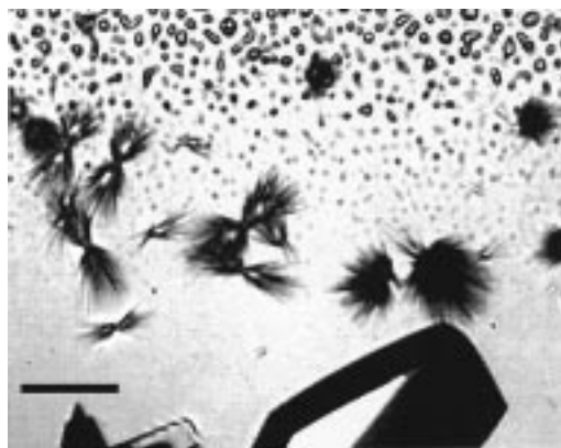
Figure 10. Selected light microscopy field showing growth of "sea-urchin" crystallites from coalescing domains under the conditions of Figure 7, 2 h after attaining maximal turbidity. The bar indicates 100 \mu\text{m} .
